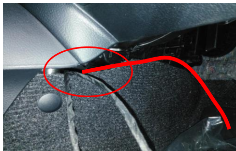
7) right motor wire and OBD line from this position to drive site
