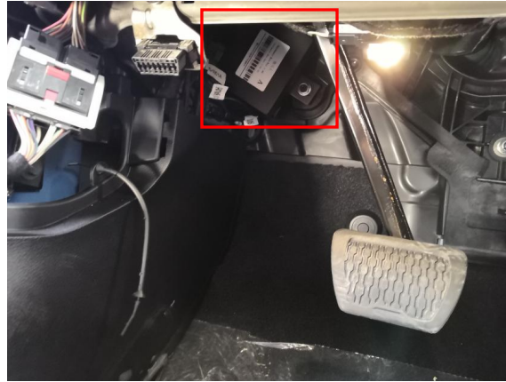
8) Fix the ECU in the driver room
