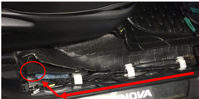
10) motor line as above position from chassis to cabin
