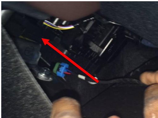
7) left motor wire from this position to co-drive site
