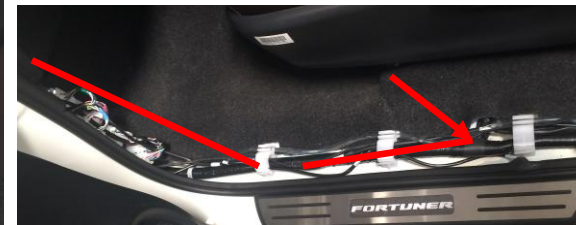
9) left motor line as above from chassis to cabin
