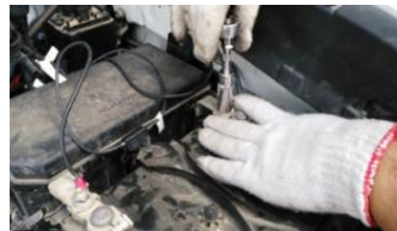
3) Caution: Tighten battery screw very tight! If loose, may get damage to the
