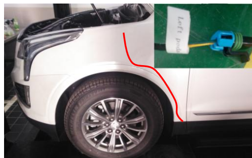
5) The left motor line as above to the chassis
