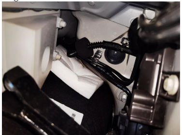
10) Turn off the original leather plug and pass through the motor wire to the chassis
