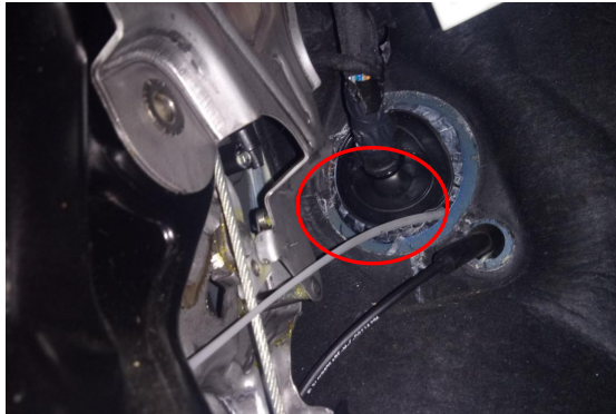
4) the positive line from here to cabin
