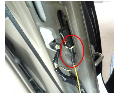
9) motor line from chassis to cabin
