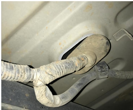
10) motor line from chassis to cabin
