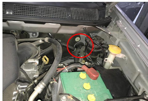
5) the positive line from here to cabin
