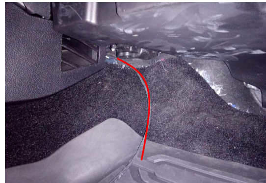
11) another motor line to co-drive side
