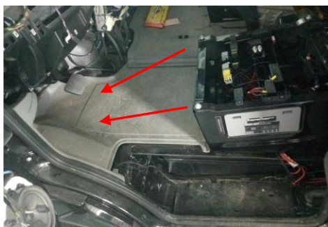
1) Lift off the co-pilot's carpet,
