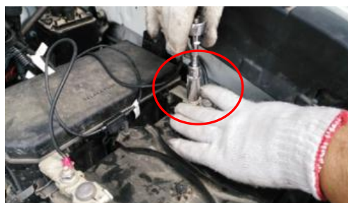
5) Connect negative pole; CAUTION!: Tighten battery screw very tight! If loose, may get damage to the car.
