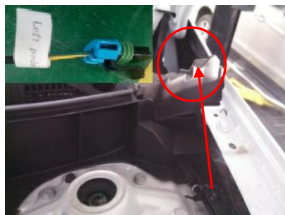
4) The left motor line is as picture position to the leaf plate
