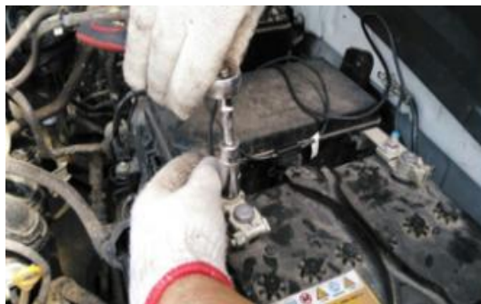
2) connect power wire to battery: red one with fuse is positive.
