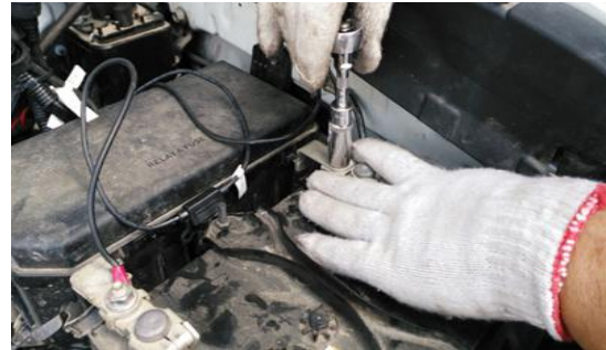
2) connect power wire to battery: red one with fuse is positive.
