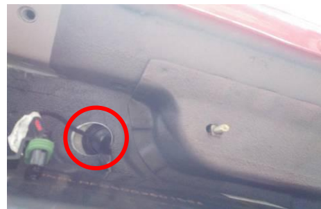
11) motor line from this hole to cabin
