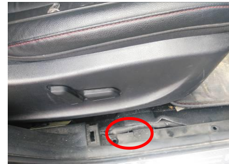
9) right motor line from above position from chassis to cabin
