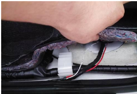
10) motor line from above position from chassis to cabin
