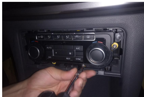
11) Remove the surrounding screws
