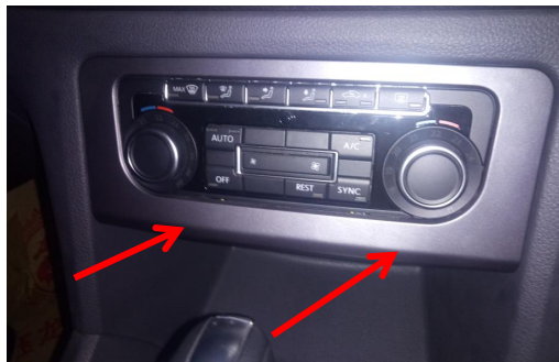
10) Pry the panel of air conditioning controller
